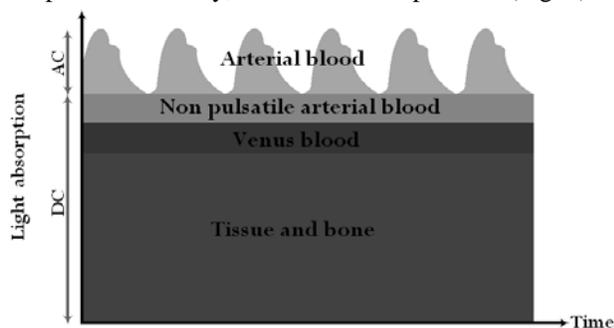
Figure 1. Pulsatile light absorption of red and infrared wavelength in human tissue.
