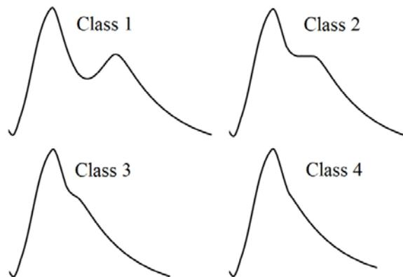
Figure 3. Standard classification of PPG waveforms.
