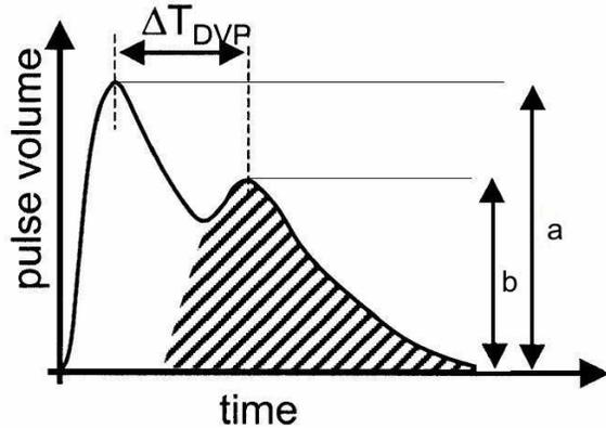
Fig 3 Depict the typical waveform of the DVP and its characteristic parameters as: time between the first and second tip ( $\Delta T_{DVP}$ ), amplitude of the first tip identified by (a), amplitude of the second tip identified by (b).
