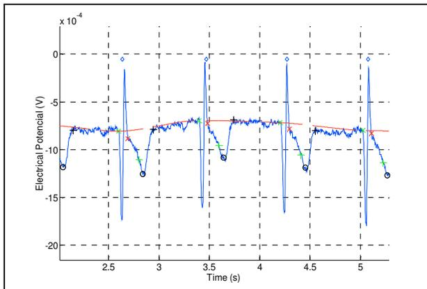
Fig.3. Detection points with our algorithm. Diamond: QRS position, Green Cross: Start QRS, Red Cross: End QRS, Circle: T wave, Green plus: Start T, Black Plus: End T, Red dash line: Base Line
