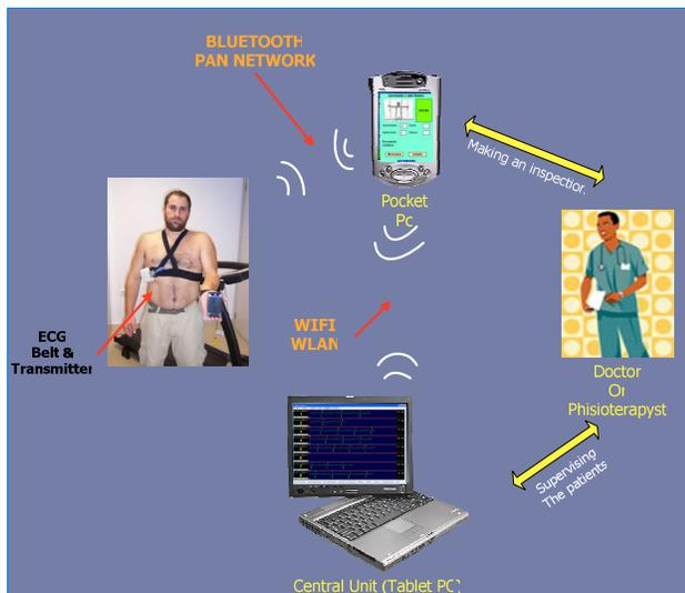
Fig1. General scheme of the system during a rehabilitation session. Two types of networks can be seen : PAN (personal area network) and WLAN (wireless local area network).
