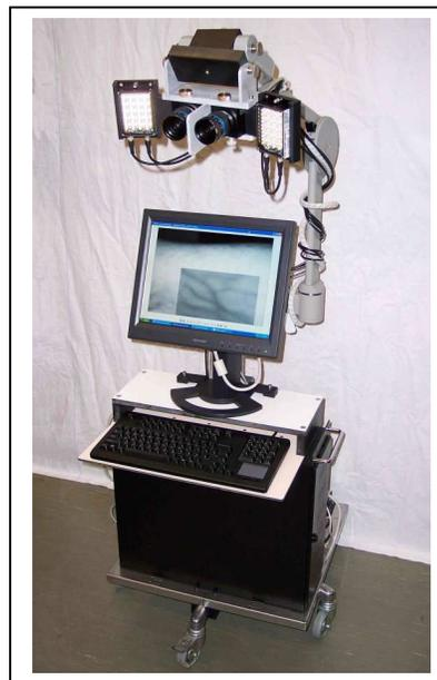
Figure 1. A trolley with the device consisting of 2 CMOS cameras plus 2 VIS/NIR LED-arrays on a swivelling arm, all connected to a dual Xeon processor PC.
