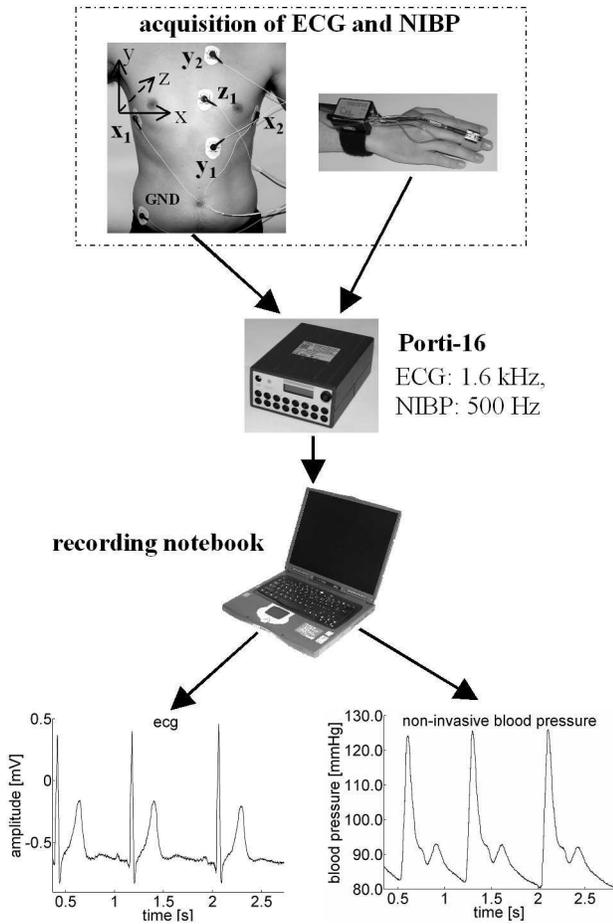
Figure 1: Measuring system for acquisition of ECG and non-invasive blood pressure.
