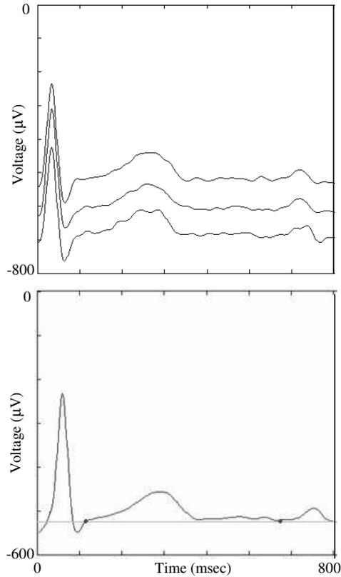
Figure 2. Example of noise reduction and improvement in morphologic shape definition. Beats of the same duration class  $QQ$  (top) were averaged in order to obtain the relevant template  $T(n)$ , from which the isoelectric line (in light gray) was identified as the intersection of isoelectric points (black dots) (bottom panel, see text for details).
