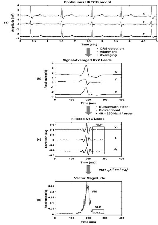
Figure 1. Computation of the vector magnitude (VM) in the temporal analysis of VLP in signal-averaged HRECG.
