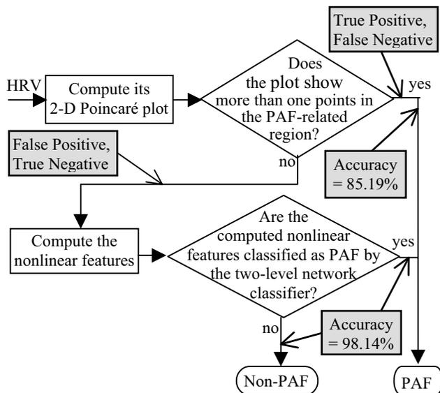
Figure 4. The flowchart of the overall system
