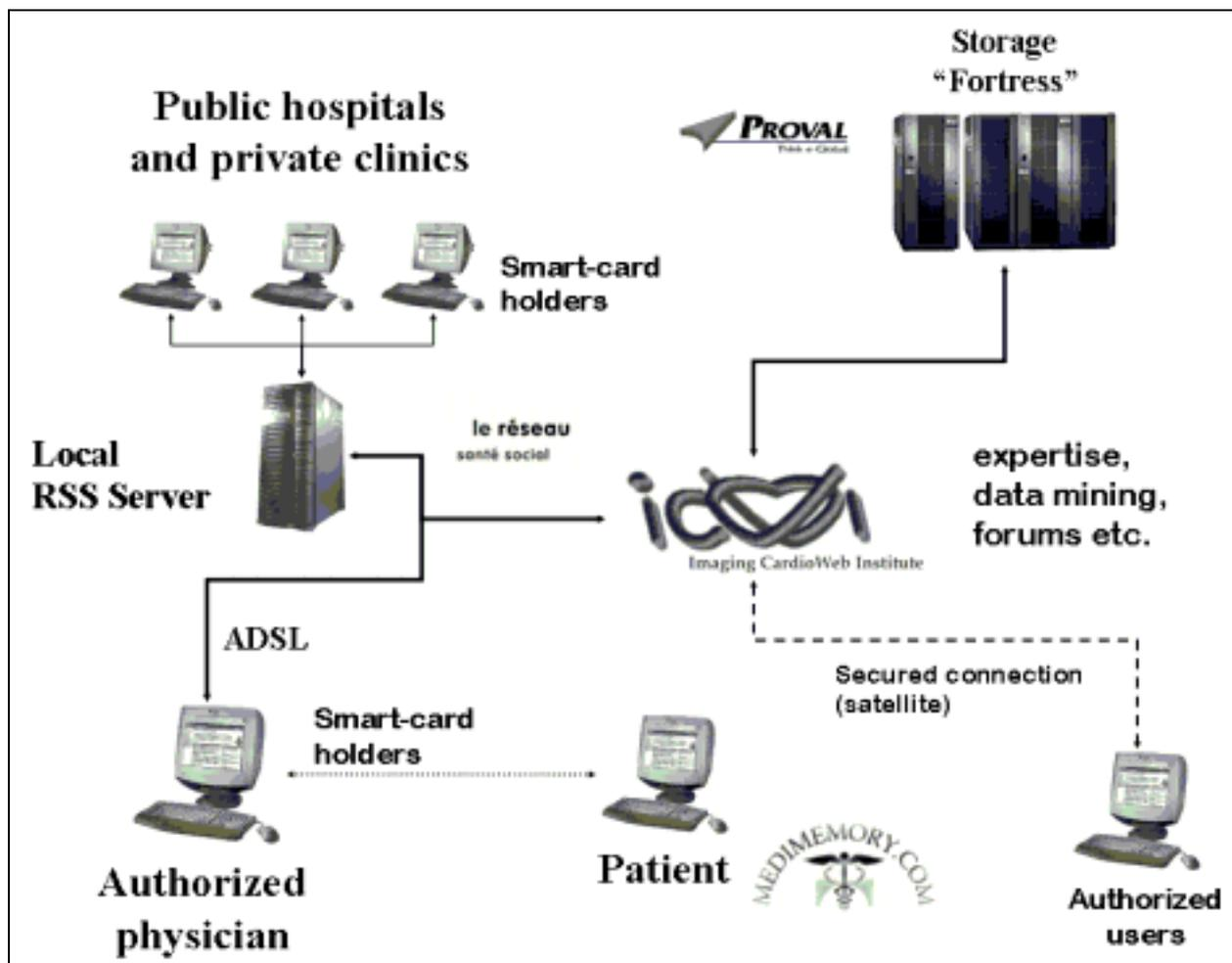
Figure 1. ICWI communications architecture.
